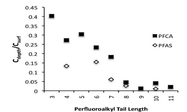
Ratios of surface concentration (Csurf) to concentration in the bottom soil core depth interval (60–120 cm, Cdepth).
