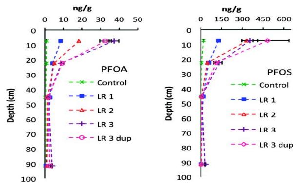
Concentrations of PFOA and PFOS with depth in the long-term plots at various loading rates.
