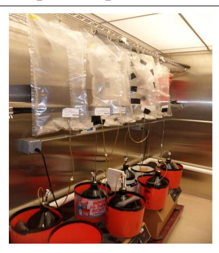
Digesters were stirred using constructed rotating chambers at 100 rpm
