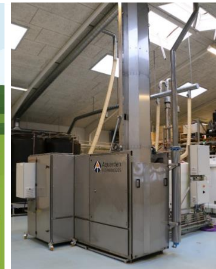
Supercritical Water Oxidation Process (Battelle's PFAS Annihilator)
